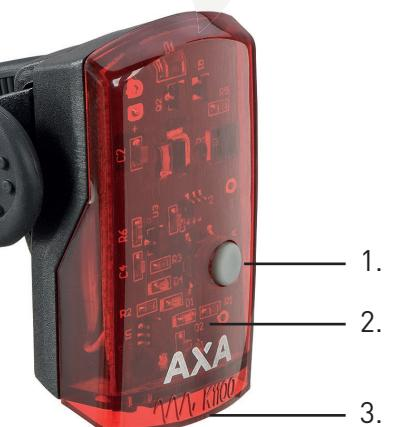
a computer. During charging, a red LED indicator (2.) shows that the light is still charging. After charging, a blue LED indicator lights up (2.). Battery indicator If the battery has reached a capacity of less than 20%, a red LED (2.) indicates that the light still has to be charged.
